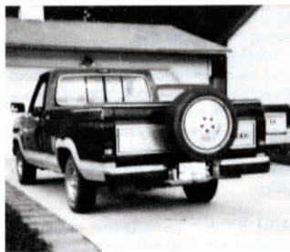
Bracket can be adjusted to fit any size tire. Bolts securely to bumper.
