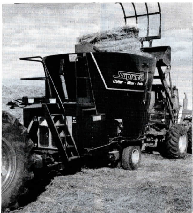
The Supreme mixer can handle loose hay or straw as well as conventional square and round bales. It thoroughly processes a batch on-the-go in 7 to 10 min.
