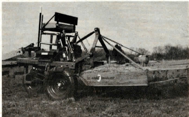
Ground-driven pto turns 3 pt. rotary mower at 540 rpms when horses move at 3 mph.
