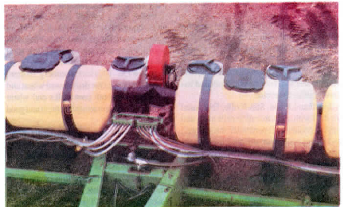
White blower mounts at center of Deere planter. Drive sprockets were reversed on each Deere row unit to accommodate air system.
