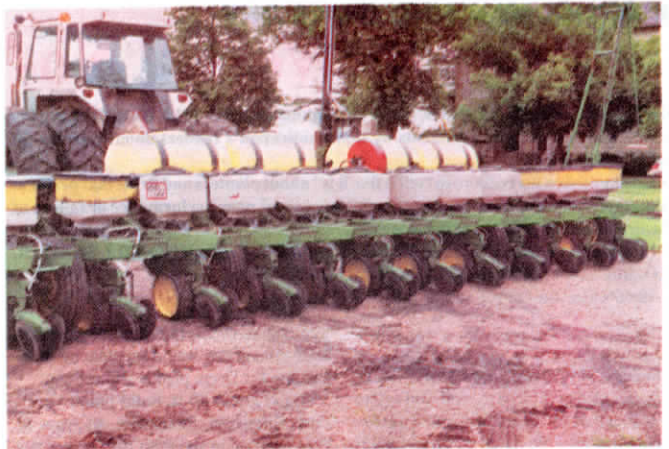
Fluhrer mounted White seed hoppers, pickup units and air delivery system on his Deere 7000 planter. "Gives me the best of both worlds," he says.
