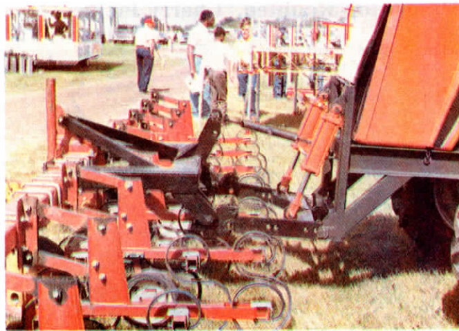
Push-pull hitch (in black) lets you push rear-mount cultivator ahead of tractor without modification.
