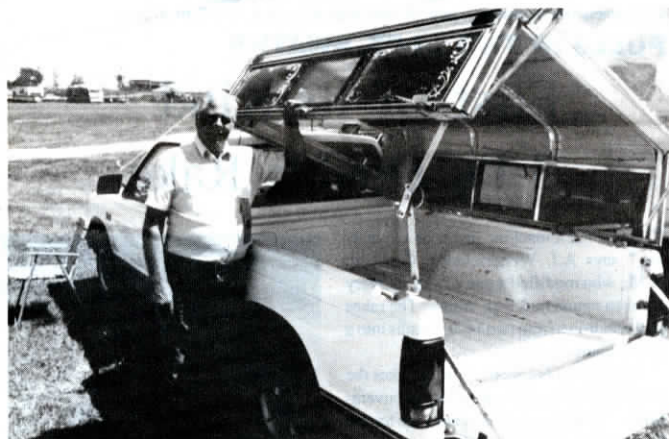
Moe's "lifters" raise either side of topper 2 1/2 ft. for easy access to entire pickup bed.
