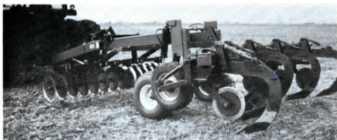
Two hydraulic cylinders raise and lower caddy. A third cylinder controls disk gang.
