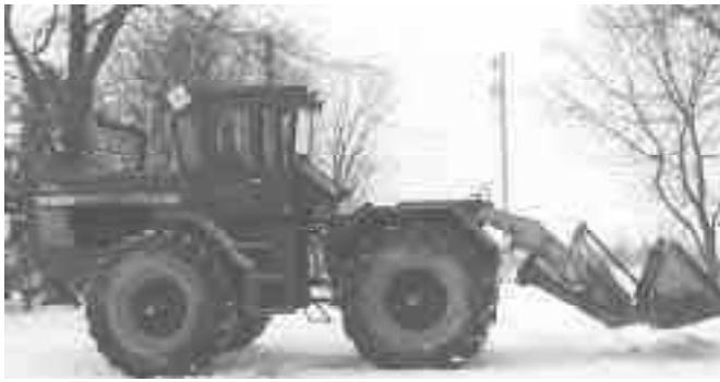
Russ reversed direction of travel on the International 4366 4-WD he uses as a loader.
