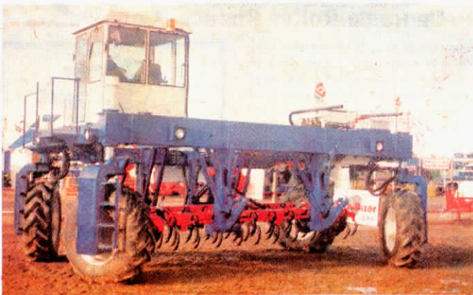
Three separate 3-pt. hookups carry implements beneath the frame of new Israeli tractor.
