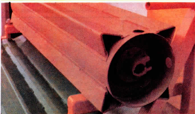
Sweco replaces lighter, 14 ga. factory paddles on Deere beaters with heavy 7-ga. beaters that weld over "stubs" of old paddles.
