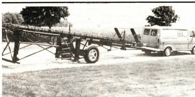
A hitch attaches to the drive-up end of the ramp so Ogram can easily park it out of the way when not in use.
