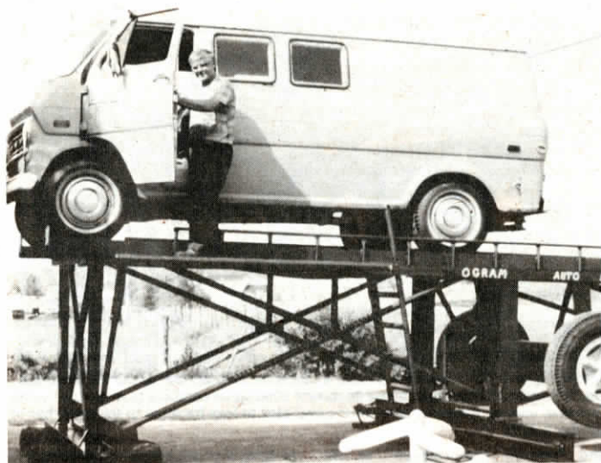
As truck drives up ramp and crosses pivot point, right, the front-end of the ramp drops to the ground, raising the ramp wheels off the ground (far right in photo).
