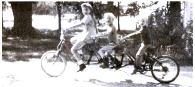
Fletcher's children love to ride one-of-a-kind bike. Middle rider controls gear shift and front and rear riders each control set of brakes.
