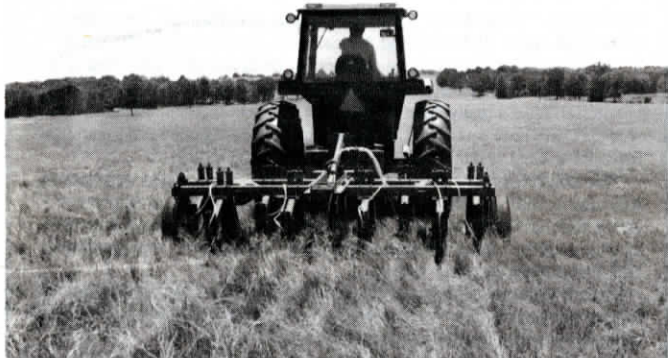
Agri-Vator is equipped with 15-in. long shanks that penetrate as deep as 8 in.
