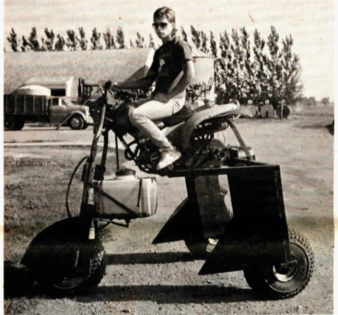
Elevated ATV rig converts back to regular use in minutes, according to Jorgenson.
