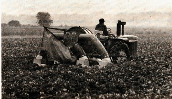
Vacuum fan sucks bugs up into 4-row machine through large plastic tubes.
