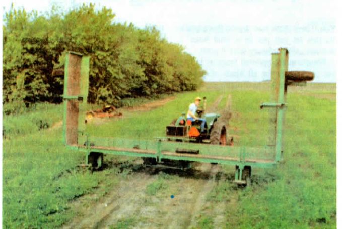
Rock-picking platform folds for transport and also dumps hydraulically to the rear.
