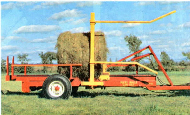
Up-front hydraulic push arm moves each bale to the rear as it's loaded.
