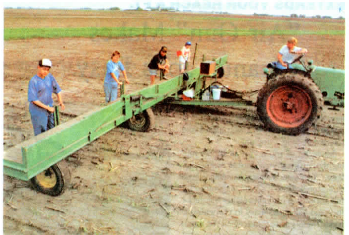
Workers ride on steps at rear of platform, hopping down to pick up rocks as they spot them. “By standing instead of walking, kids can work 8 or 9 hrs. a day without tiring,” says the farmer-inventor.
