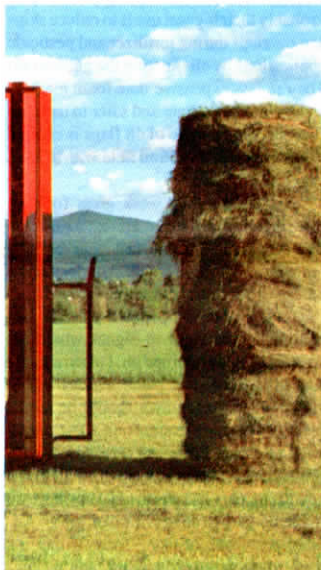
Bale-carrying platform tips up 90° to stack bales vertically.
