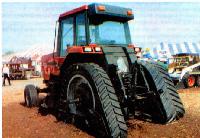
Christianson tracks fit over standard tractor tires and are held in place by side plates fitted with rollers that ride against wheel rim. (Photo shows 16-in. wide tracks on one side of tractor and 30-in. wide tracks on the other.)
