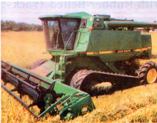
Rear steering wheels are held off ground when traveling in a straight line but drop down automatically when operator touches steering wheel to make turn.
