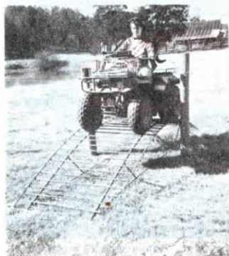
Concrete reinforcing rod was welded together to make the 2-ft. high ramp.
