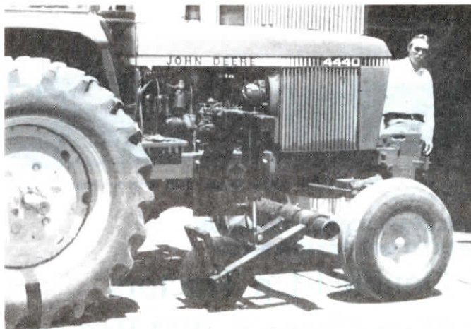
Sharp-edged wheel makes a furrow that's 7 to 9 in. deep and 5 in. wide. Furrow is easy to follow with single rib tires on tractor and guidance wheels on cultivator.
