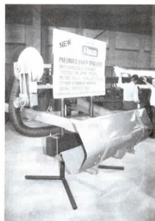
New chaff spreader blows chaff out in a wider and more uniform spread than spinner-type chaff spreaders.
