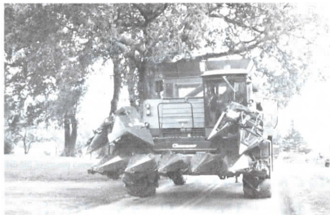
The Geringhoff header, which is the first folding cornhead in North America, features shredder-rollers that replace the snapper rollers.
