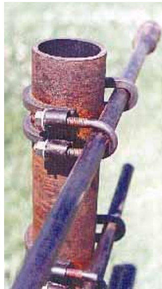
Horseshoe-shaped clamp is made from 3/8-in. sq. steel bar and allows steel rods to be secured to fence posts made from common 2 7/8-in. dia. round tubing.
