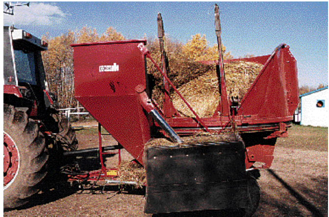
Add-on grain hopper mounts on front of a Case-IH 8610 big bale processor. A 4-in. dia. auger lays grain on top of the hay which is laid down in a windrow.
