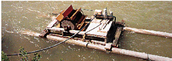
Floating pump consists of a piston displacement pump mounted on pontoons that were made from two 15-ft. lengths of 6-in. dia. irrigation pipe.
