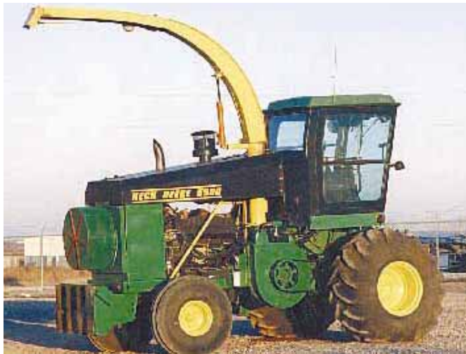
The "Keck/Deere 5950" features an 855 cu. in., 400 hp diesel out of Kenworth semi.
