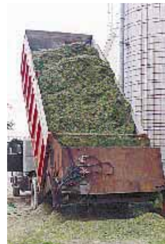
"Blower deck" delivers silage into a silage blower.
