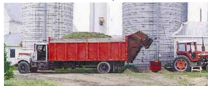
Truck is equipped with a 21-ft. long, 8 1/2-ft. wide, 6-ft. high home-built steel box.
