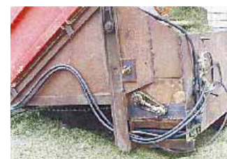
Deck is equipped with orbit motor-driven floor chain, beater, and rubber conveyor.
