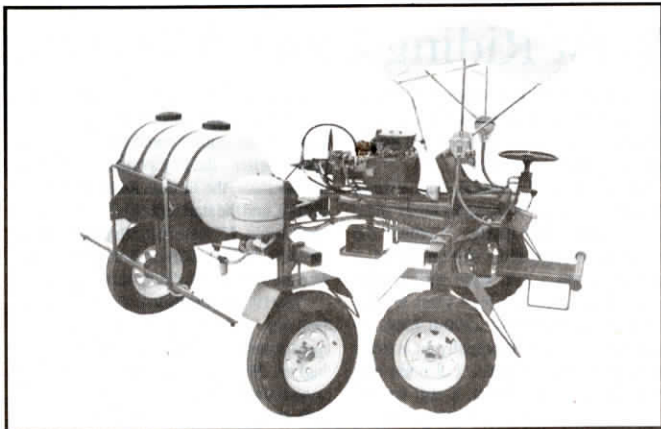
"Spider" articulates in the middle, giving it an 18-in. turning radius.
