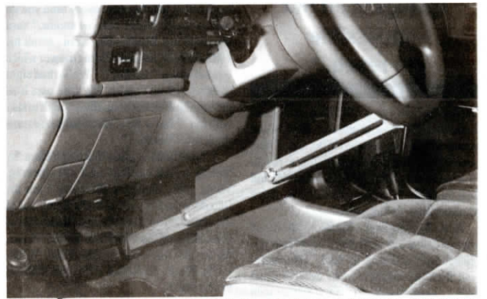
Idlestick is made out of oak and unfolds like a fold-out wooden ruler. Works great when jump starting a dead battery to maintain a high charging idle.
