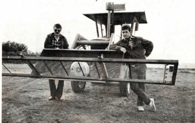
Hopper killer consists of a 2 by 12-ft. metal grid that mounts on a tractor front-end loader.
