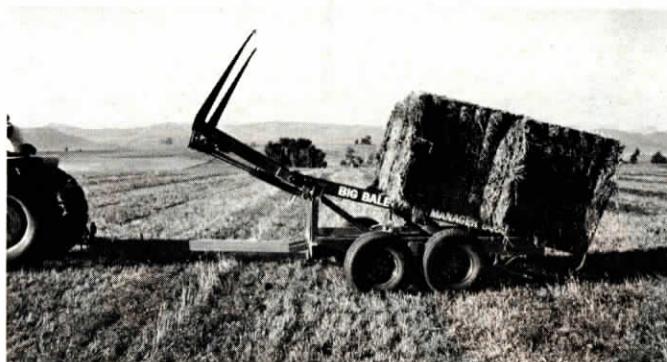
Up-front bale forks load bales onto inclined bed of carrier. They slide to the back by gravity.
