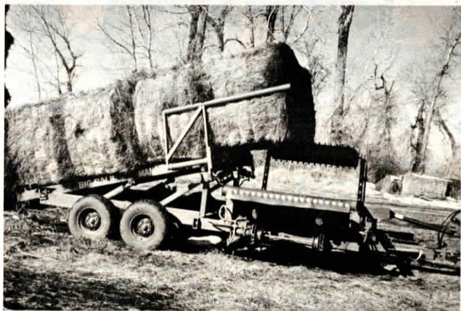
Bale feeding mechanism is mounted in place of bale-loading forks at the front of the Bale Manager to feed bales out to livestock.
