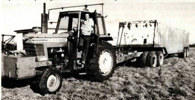
Pto-driven semi-truck grain hauler has air brakes that are activated by air compressed with an old air conditioning compressor that mounts on the trailer tongue and is driven by the trailer's transmission.
