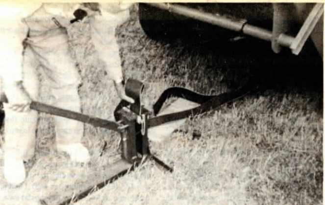
With one motion the portable Lever Lacer squeezes the laces tight enough to clinch the teeth.
