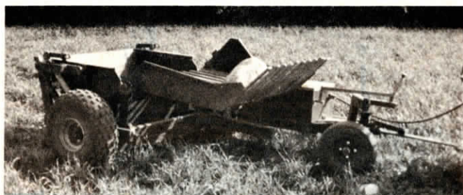
The new ATV rockpicker handles rocks up to 500 lbs. Front fork lifts rocks into rear dump bucket.
