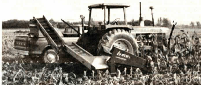
New tractor-mounted one-row picker dumps into a tag-along wagon or drive-along truck.
