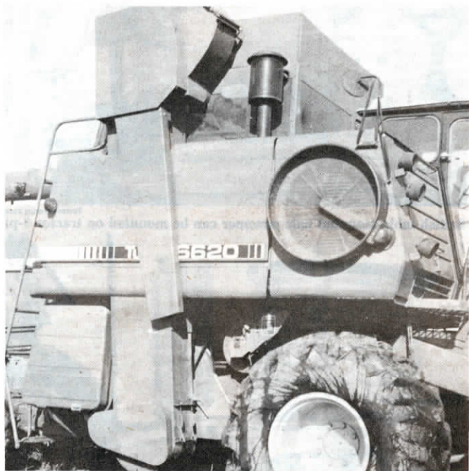
Add-on elevator increases combine grain handling capacity.
