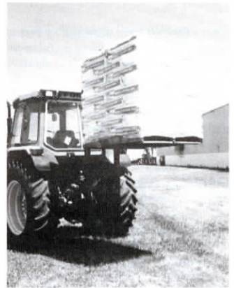
New tractor forklift can handle a pallet load of as many as 66 bags of seed.
