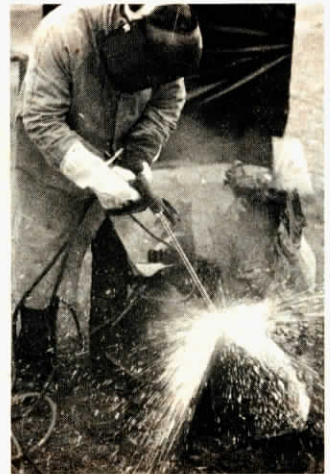
Oxygen and 12-volt electricity fuel cutting rod that simply slips into end of torch.
