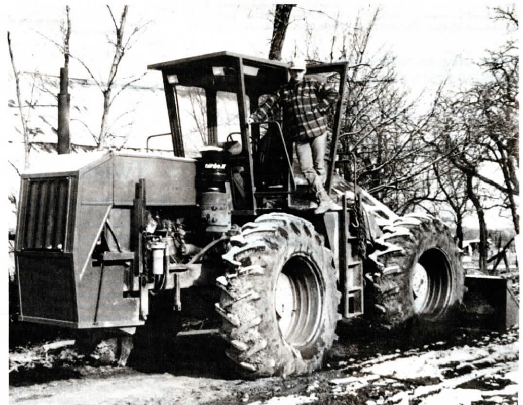
The tractor was built with the drive axles and transfer case from an industrial front-end loader and a 15-speed transmission from a semi truck. The frame was fashioned out of 9 by 2-in. solid steel bars.
