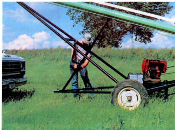
Mover mounts on auger axle. Tongue attaches to hitch on pickup bumper.
