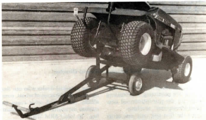
Hand-operated lift easily raises mower, or other equipment, 2 ft. or more off the ground.
