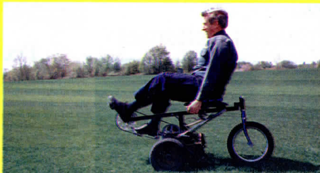
Pedal-powered mower can cut about as much grass as a medium-sized gasoline-powered push mower, according to the inventor.
