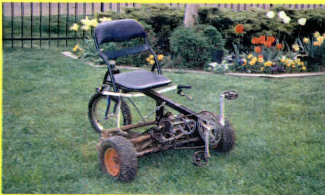
The reel-type mower cuts a 26-in. swath. It steers via cable connected to modified bicycle handlebars mounted under seat.
