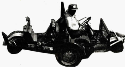
Kashubara's home-built car has small turning wheels front and back and two full-size wheels at center.
