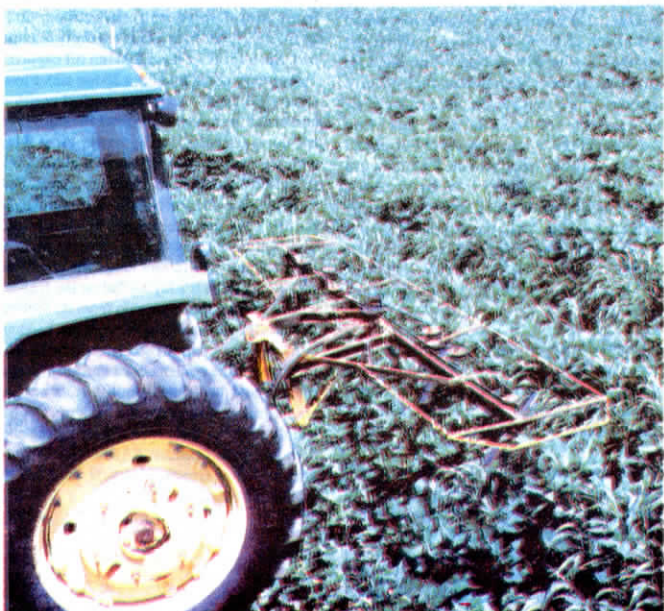
The 10-ft. wide weed "topper" is equipped with five 30-in. blades.
