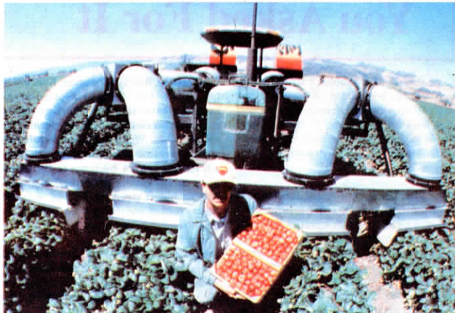
Bugs are sucked up through the air ducts and right into the fan blades which pulverize the bugs and blow them back onto the field.
