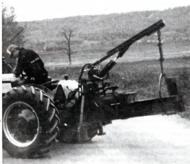
The 4 1/2-ft. long boom is fitted with a clam-type log lift which works like a pair of ice tongs.
