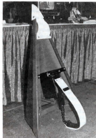
Note plastic point and skid shoe on point of snout. May-Wes sells this point assembly, which bolts into place, for $20 to fit Case/IH cornheads (800, 900 and 1,000 series), Deere quick-tach heads, and Gleaner "black frame" heads. The bowed skid shoe keeps the point about 1 1/2 in. above the ground.
