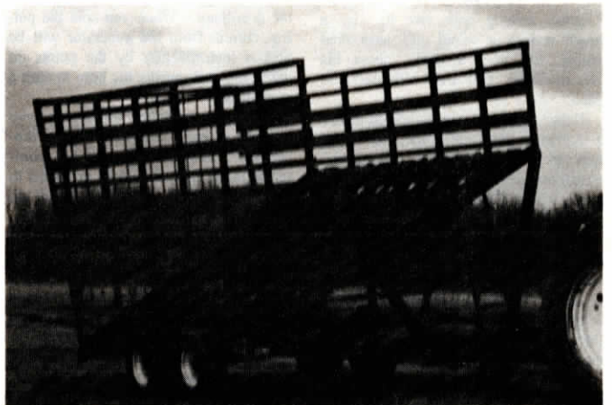
"Handy Dump" is sloped to self-unload 140 bales in 30 seconds.
