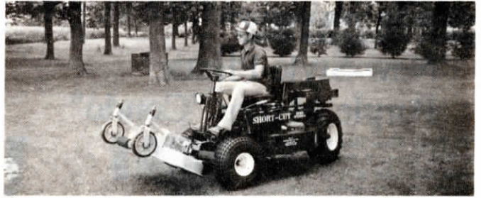
Hydrostatic drive on steerable single rear drive wheel powers the mower.
