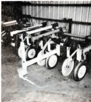
Front sensor uses wand to sense position of plants in row.
