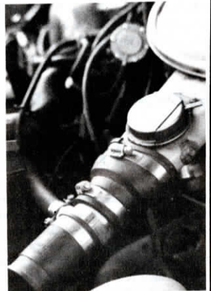
Propane valve attaches to air cleaner. Gas control valve is at upper part of photo.
