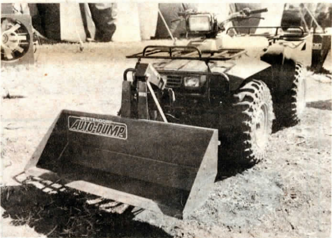
Loader and electric lift can also be adapted to most garden tractors.
