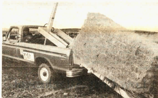
Bale carrier extends out and under bale. Drag chains pull it into pickup.
