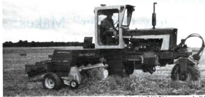
Fry combined a 1971 New Holland pull-type baler with a 1967 IH 706 tractor to build the baler. A flotation tire in front, powered by a hydraulic motor, pulls the rig.
