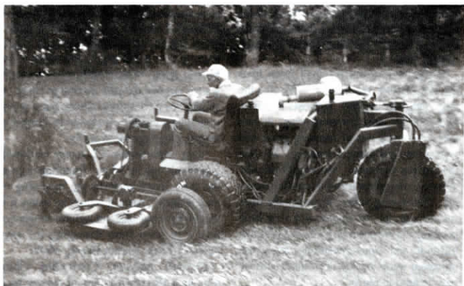
The three 3-ft. mower deck sections are supported in front by three 12-in. caster wheels and in back by four 13-in. car wheels. A pair of 8-in. rubber wheels on each outside section of deck serve as "bumper guards".
