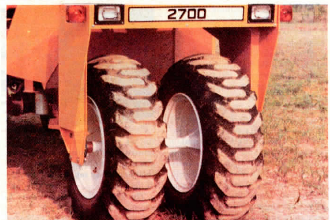
Two-wheel row crop wheel kit replaces standard wide flotation tire found on most "floaters".
