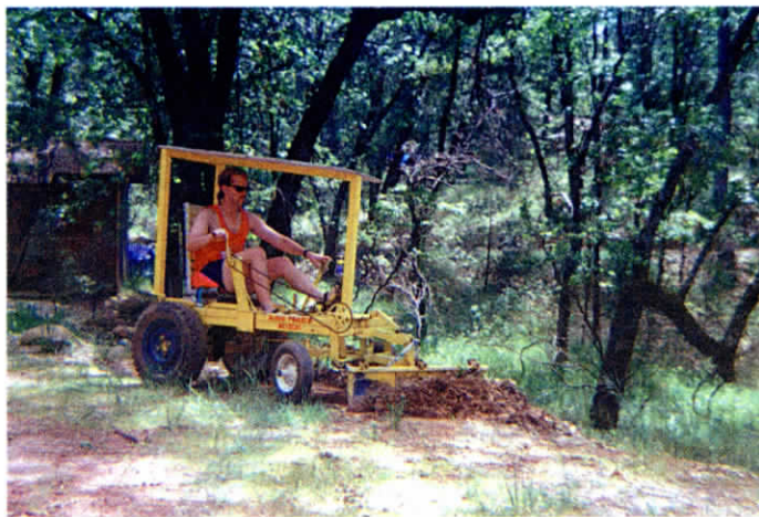
Pedal-powered bulldozer is driven by a bicycle chain and sprocket and 5-speed transmission. Bike chain and sprocket drive on right side turns by hand to control height, tilt and pitch of the 3-ft. wide blade.
