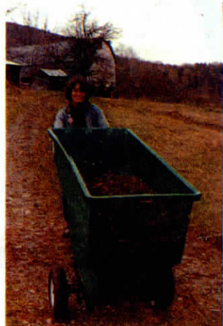
Bin is dumped by hand or can be decoupled from the 3-wheeler to be used as a wheelbarrow.
