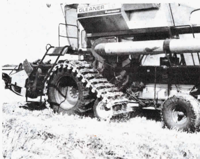
All-steel Loegering tracks, shown here on a Gleaner, fit most combines and cost $7,000 to $9,000 per set.
