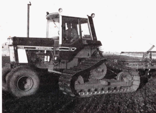
The Piepers, of Iowa, offer a "package" for equipping tractors, combines with D-5 Caterpillar tracks.
