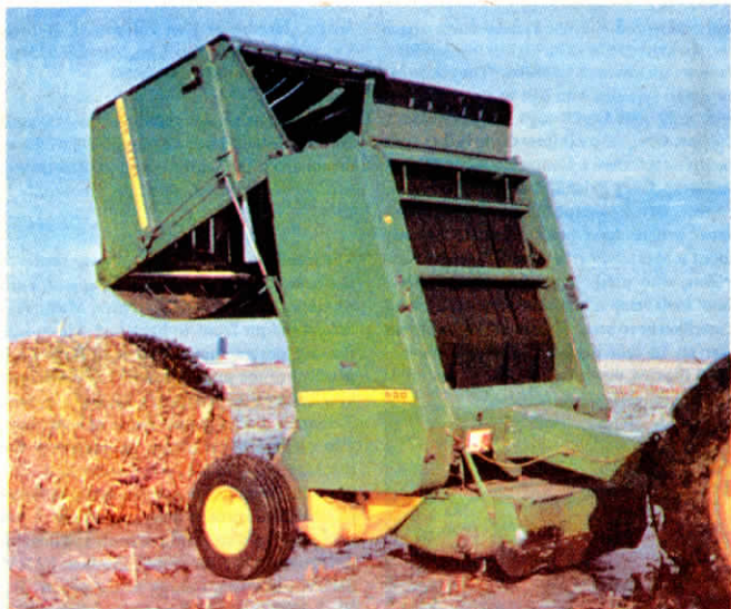
Chopper mounts in place of hay pickup and is belt-driven at 1,400 rpm's off the main baler drive.
