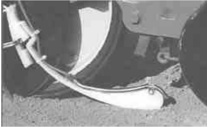
Curved 8 1/2-in. long stainless steel tube attaches by means of a plastic fitting to any conventional liquid tube. To mount it you drill a hole through the seed firmer and then rivet a metal tab into place.
