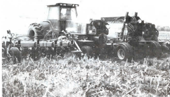
Bolt-on tool carrier moves tractor's front wheels and axles forward 15 ft. A 12 by 12-in. steel toolbar carries planter or cultivator.
