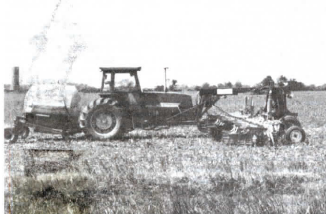
Eppley pushes a 16-row Buffalo cultivator, pulling a 1,000-gal. spray tank behind.
