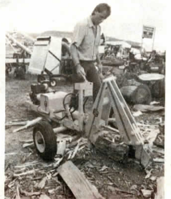
Engine-driven hydraulic pump is available for remote or trailer-mounted operation.
