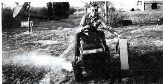
The washer lets you clean out under the mower deck without getting off the tractor by simply driving over the water jets, turning on the water and starting up the mower.
