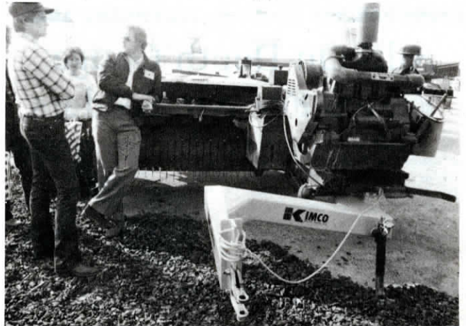
Offset hitch allows both tractor and baler to straddle windrow.
