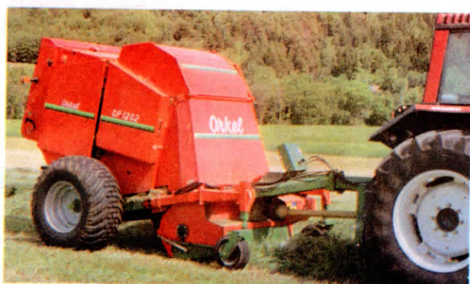
Up-front chopper, fitted with 18 rotating knives, picks up, chops and blows crop material into bale chamber. It lets you pack 30 percent more material into a bale.
