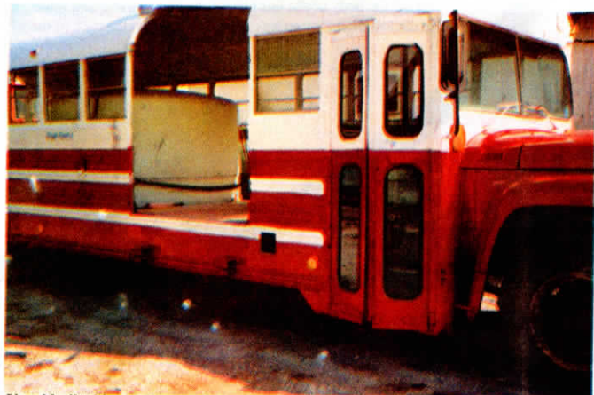
Vogel built this planting and spraying supply truck by cutting the back and side off a bus and putting a 1,000-gal. nurse tank inside.
