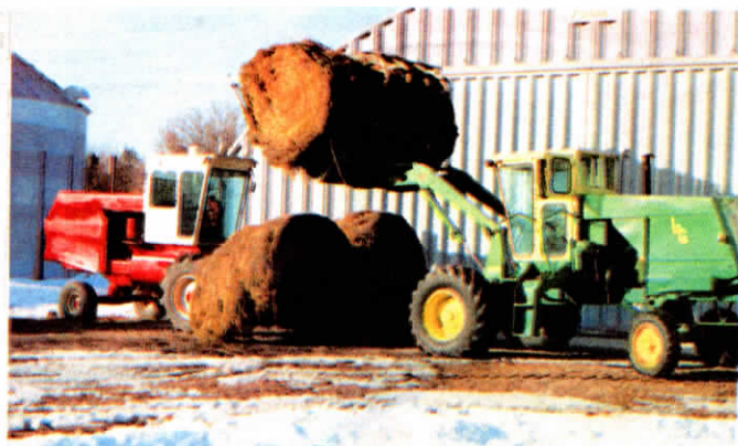
After reading about the idea in FARM SHOW, Bill Leiser converted Deere and IH combines into loader tractor. He built them for less than $4,000 apiece.
