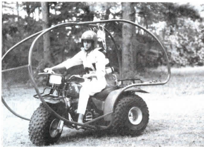
Cage is equipped with a safety harness that holds rider safely in place as machine rolls.
