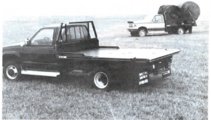
Pickup box is replaced with a "Hydra-Bed" to let you pick up, haul and unroll bales.
