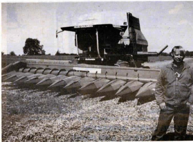
Barnett used this Gleaner combine to set record (photo shows bean head, not corn head). The only modification he made was to boost grain tank capacity to 370 bu.
