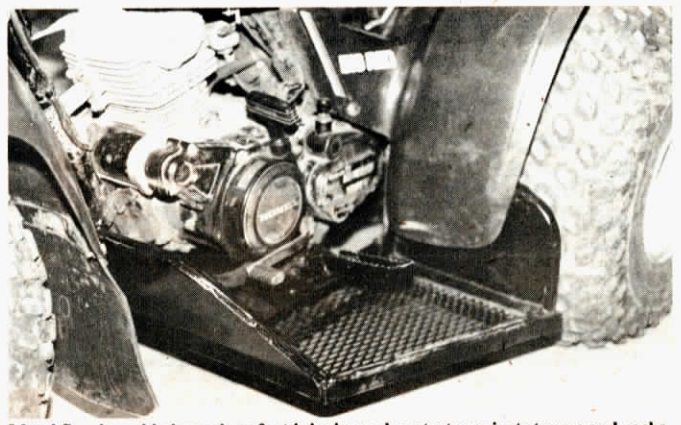
Metal floorboard helps reduce foot injuries and protects against stumps and rocks.
